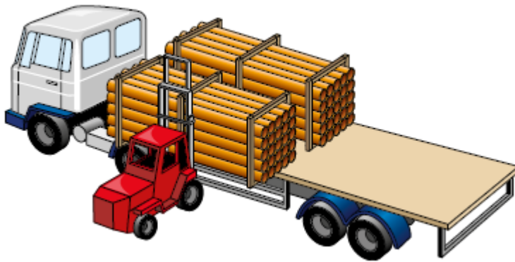
Figure 12: Loading block bundles on to flat bed vehicle
